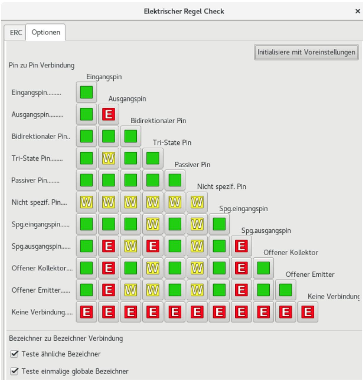
Rules can be changed by clicking on the desired square of the matrix, causing it to cycle through the choices: allowed, warning, error.
