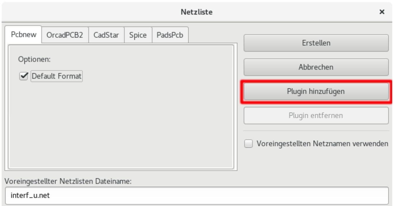
New generators require a name and a command. The name is shown in the tab label, and the command is run whenever the **Export Netlist** button is clicked.
