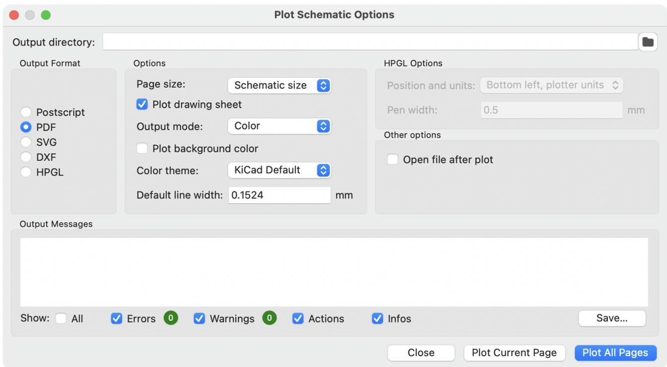
The **Output Messages** pane displays messages about the generated files. Different kinds of messages can be shown or hidden using the checkboxes, and the messages can be saved to a file using the **Save...** button.
