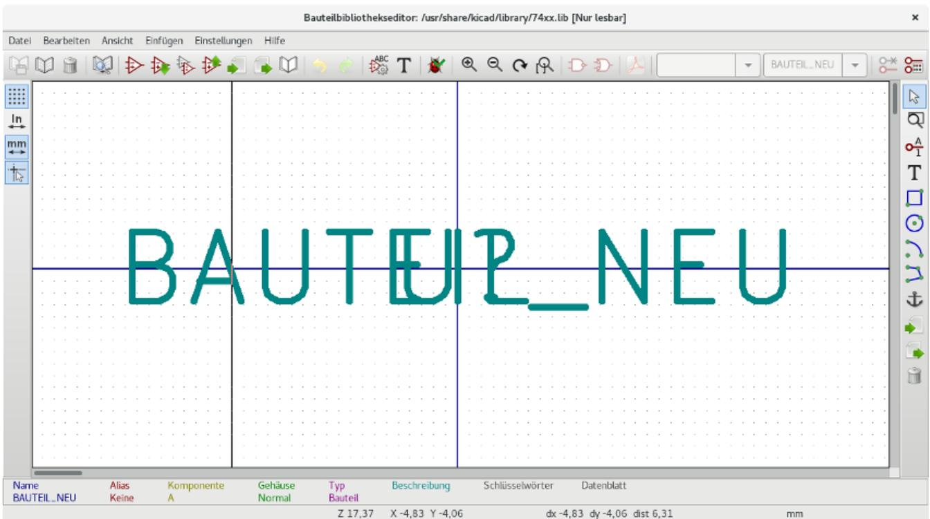
The blue cross in the center is the symbol anchor, which specifies the symbol origin i.e. the coordinates (0, 0). The anchor can be repositioned by selecting the
